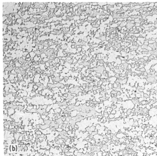
Figure 4 Optical micrographs of two-phase Mg–Li alloys. (a) Mg–5.5% Li (I-29); hot-rolled and then cold-rolled 40% to t = 0.9 mm followed by annealing at 300°C for 1 h. (b) Mg–7.5% Li alloy (I-12); hot- and cold-rolled to t = 1.1 mm and then annealed at 300°C for 1 h. (c) Mg–9.5% Li alloy (I-17), cold-rolled 90% to t = 0.8 mm and then annealed at 300°C for 1 h. ( \times 100 ).
